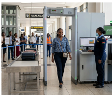
1. Personal Screening Walk-through metal detector detects concealed metal objects
